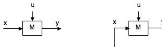
Figure 4: Schematic of Operationally Open System (Left) and Operationally Closed System (Right)
