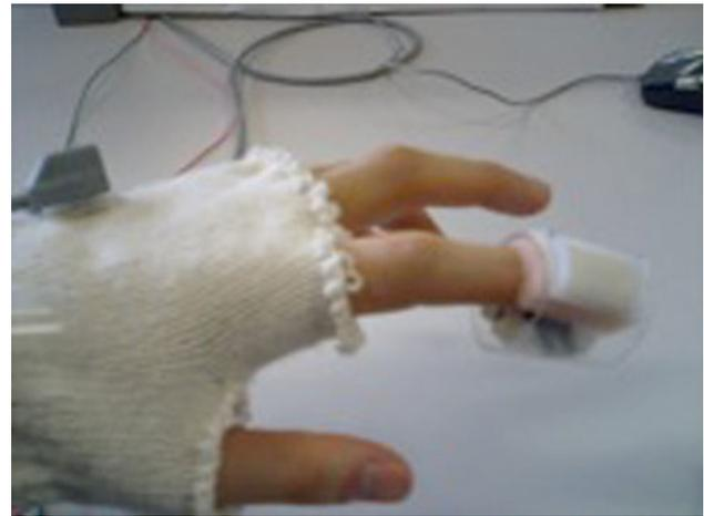
**Fig. 7** Picture of the active tactile system as it is being worn by a participant. The 3D position sensor is visible on the back of the hand, and the ICPF-based tactile display is visible on the tip of the index finger [96]
